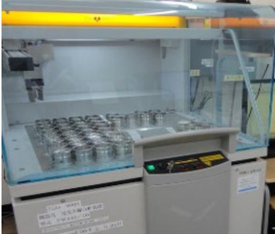
**Model Name: PAnalytical X-ray fluorescence spectrometer Axios mAX system**
