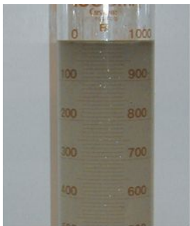
Rolling oil after removing ferrous particle
